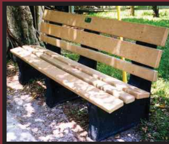
Bench constructed of recycled plastic lumber
